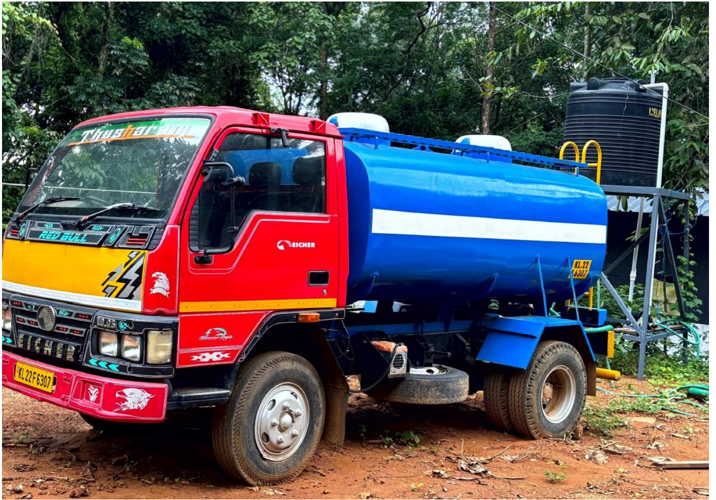
Dust Suppression water tanker
